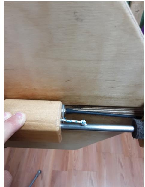
3 Cord is secured to picker with fat knot
